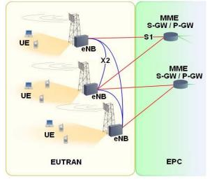
Figure 1:LTE-System Architecture Evolution(SAE)[3]
