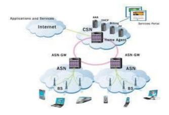
Figure 2: Mobile Wimax Network Architecture[6]
